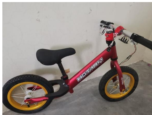
Fig. 5. Assembly of 3D Printed Handlebar on Hotaru Balance Bike
