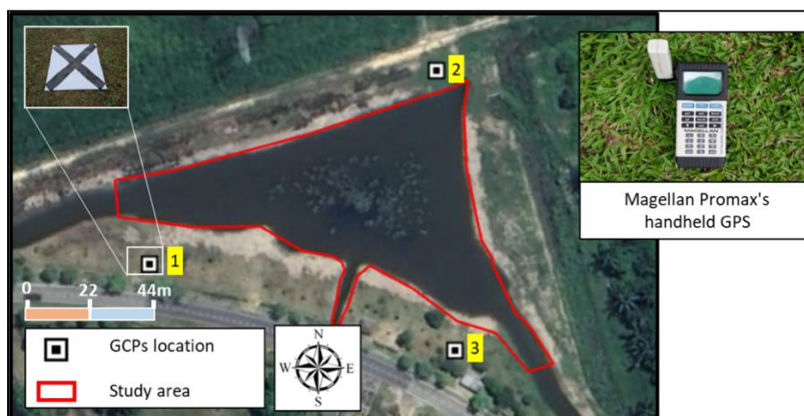
Fig. 3. Ground control points locations
