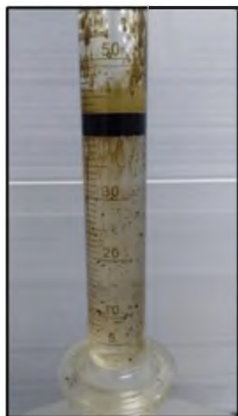
Figure 13. Oil extracted after water and polymer flooding at 60 °C. The polymer solution consisted of 2000 ppm of HPAM and 0.8 wt.% CSNPs.
