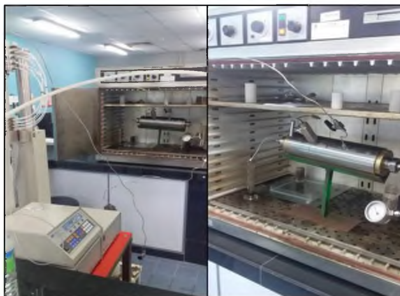
Figure 39. Main core-flooding apparatus used in experimental work.
