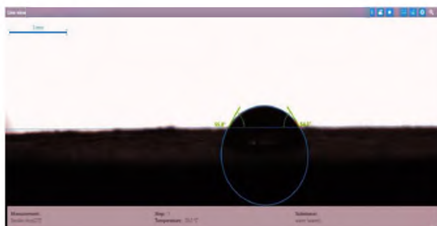
Figure 12. Contact angle for a disc of a core sample soaked in crude oil and HPAM (2000 ppm) + CSNPs (1.25 wt.%) at 60 °C.
