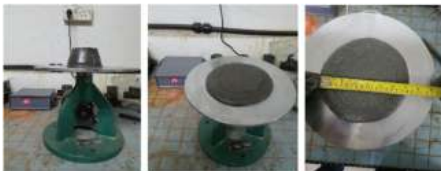
Fig. 1. Slump test of the proposed mortar.
