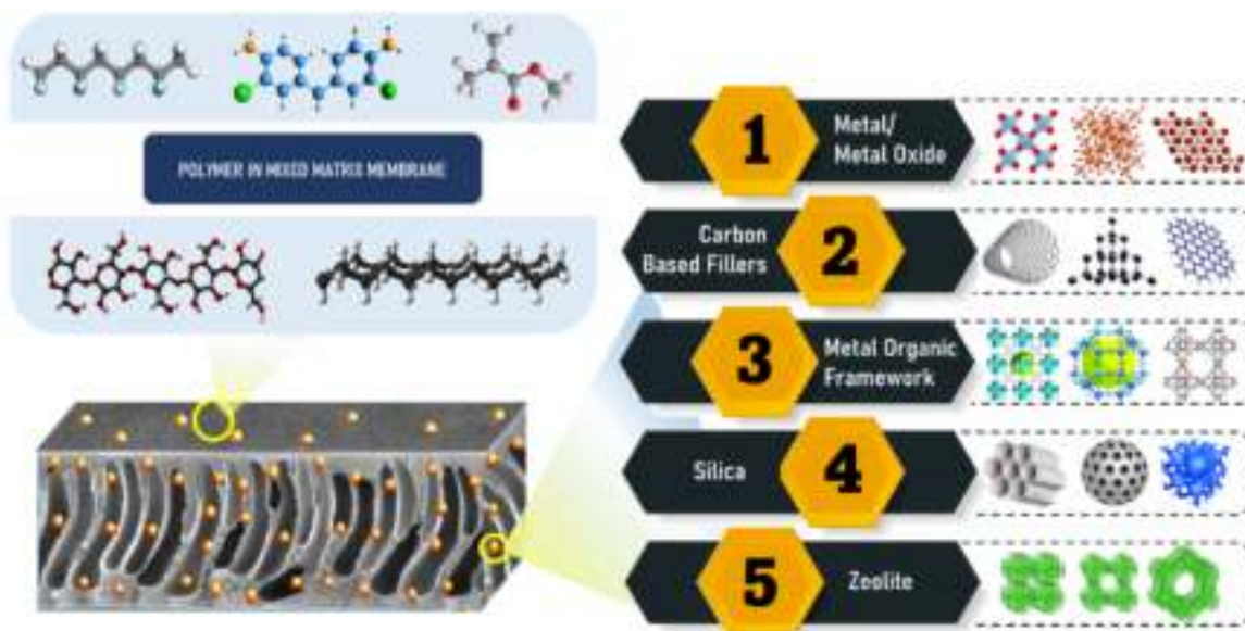
Fig. 6. MMM structure and filler in MBR
