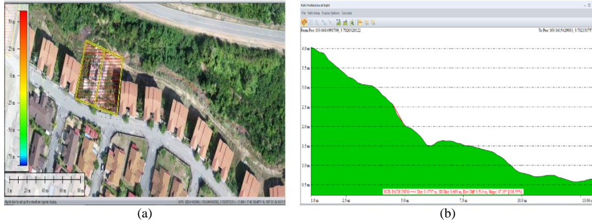
Fig. 8 - Potential slope hazard for slope A
