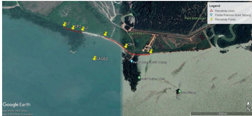
Fig. 4 - The location of resistivity line of L1 to L1’ and L2 to L2’
