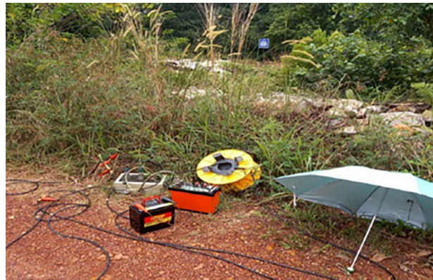
Fig. 3 - The equipment set-up of ABEM SAS 1000
