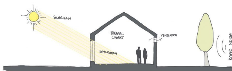
Fig. 4 - Basic building design for internal thermal comfort [12]
