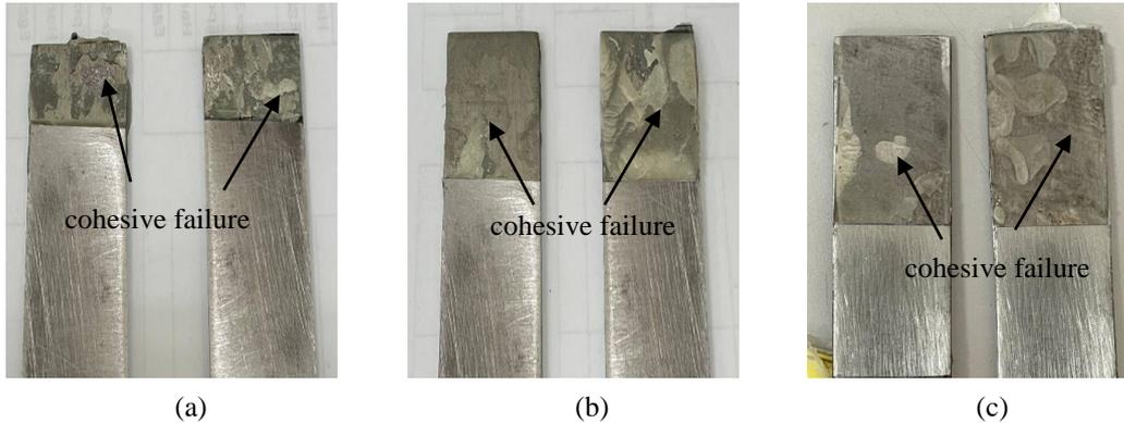
Fig. 7 - Cohesive failure in different adhesive overlap length; (a) 12.7 mm; (b) 25.4 mm; (c) 38.1 mm
