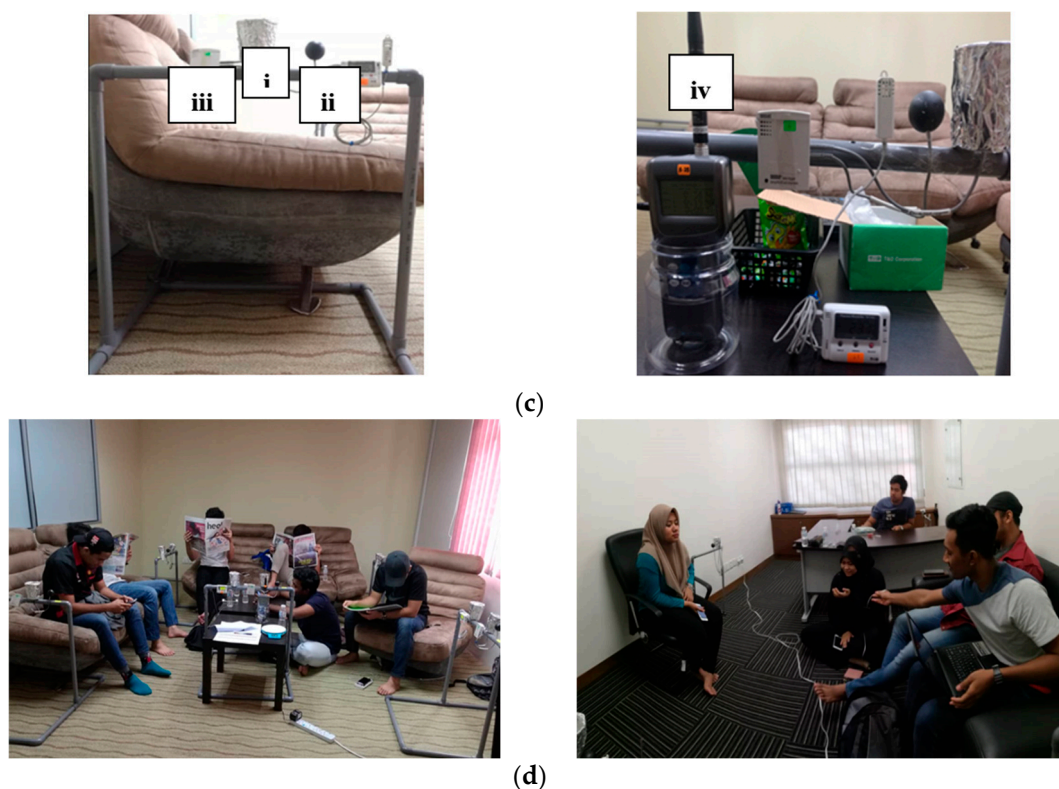
Figure 2. (a) Studied building, (b) floor layout, (c) equipment setup—(i) air temperature, T_a ; (ii) globe temperature, T_g ; (iii) relative humidity, RH ; (iv) air speed, V_a —and (d) photos of respondents in the student activity rooms.
