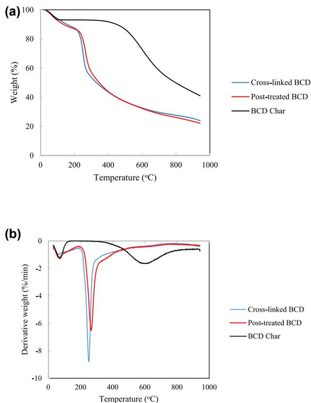
**Figure 1:** Thermal degradation profiles of  $\beta$ -CD polymers, (a) TGA and (b) DTG curves.
