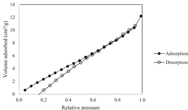
**Figure 2:**  $N_2$  adsorption-desorption isotherm of post-treated  $\beta$ -CD polymer.
