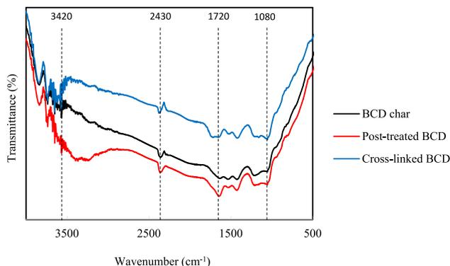
**Figure 3:** FTIR spectra of  $\beta$ -CD polymers.
