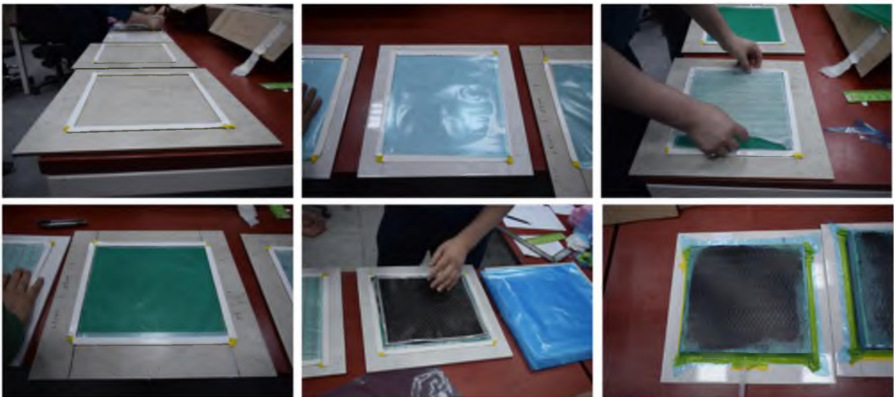
Figure 2. Manufacture of CNTRC composite material.
