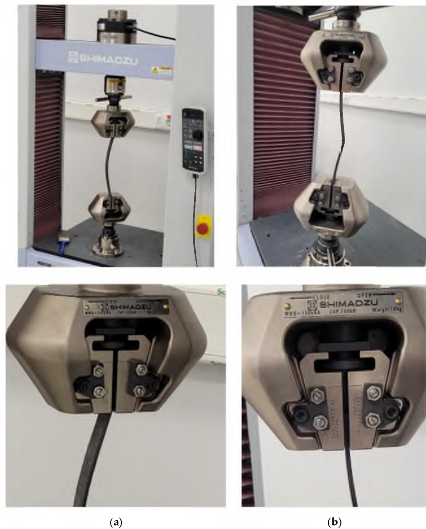
Figure 5. Test setups depending on boundary conditions. (a) simple–simple; (b) clamped–clamped.
