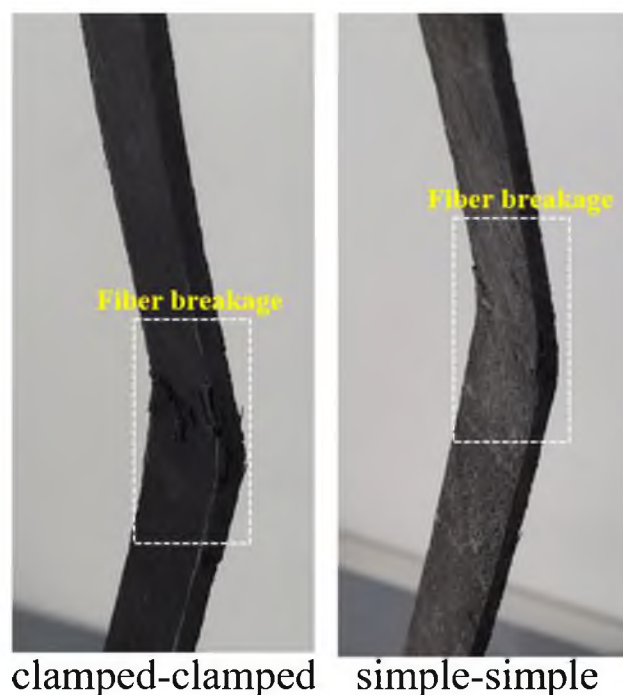
Figure 10. Damage analysis of simple–simple and clamped–clamped supported samples.
