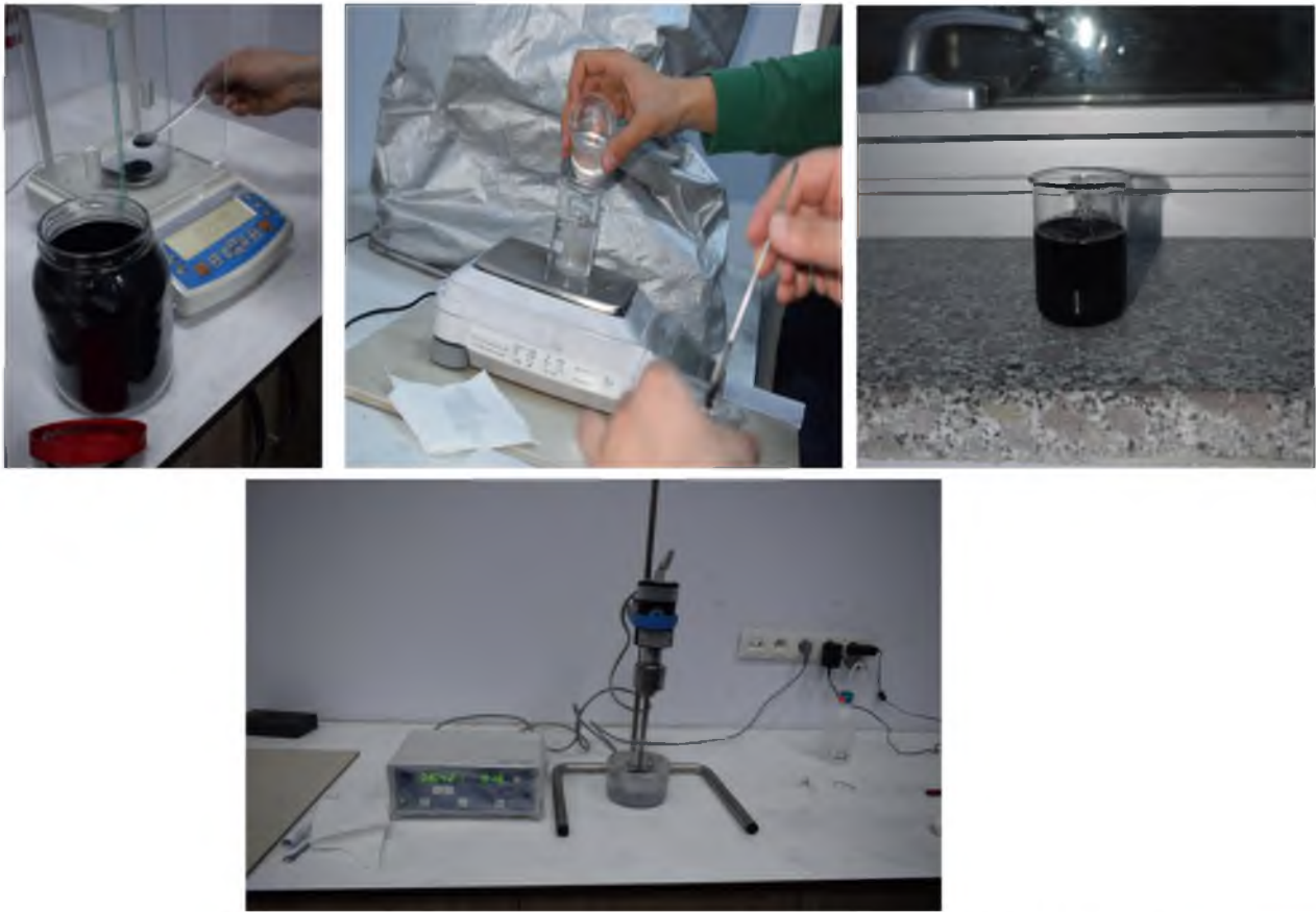
Figure 1. CNTs in epoxy resin and using the mixture of resin/CNT as the matrix of the composite.
