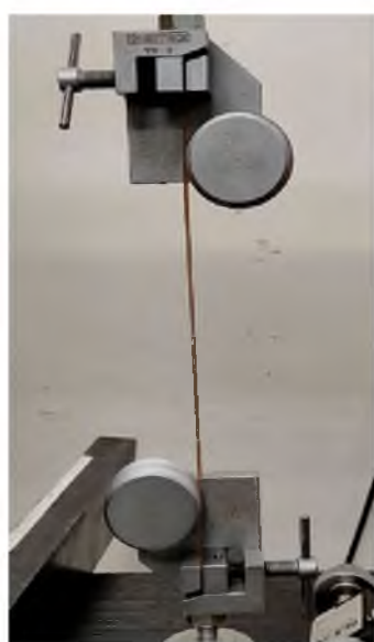
Figure 7. Wire pull test.
