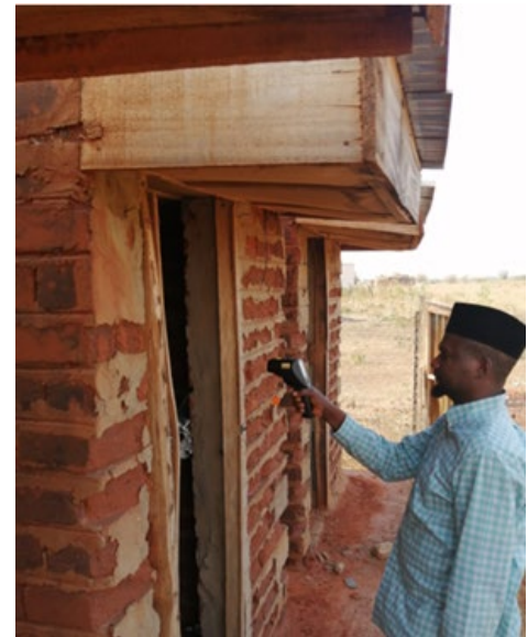
Figure 10. Testo Infrared thermometer surface temperature monitoring
