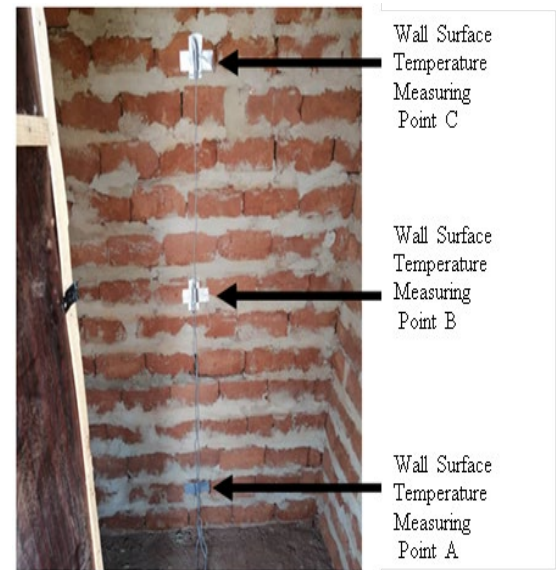
Figure 9. Internal Walls surface temperature measuring points
