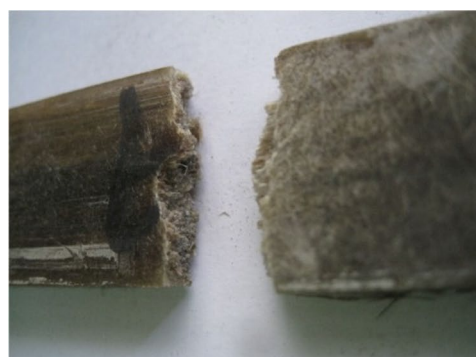
(a) Rupture section of KFRP composite sample.
