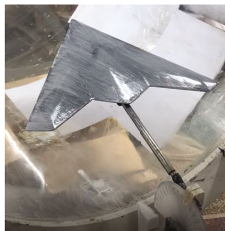
FIGURE 8: The Model installation in NCKU wind tunnel at angle of attack of 15°.
