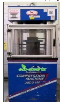
(b) Compression test on concrete cube
