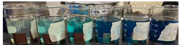
Figure 2 Immersion tests in CuSO 4 solutions
