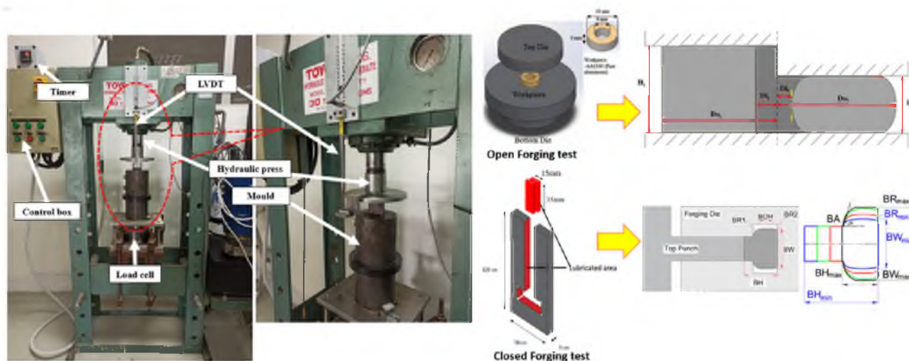
Figure 1. The open-closed forging test set up [15,17].
