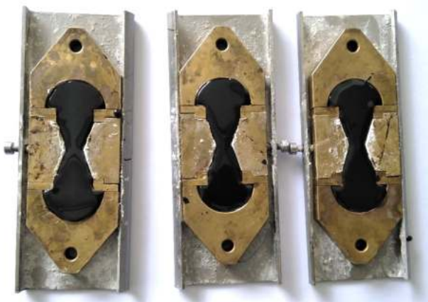
Fig. 3 Cup lump rubber-modified sample prepared for ductility test
