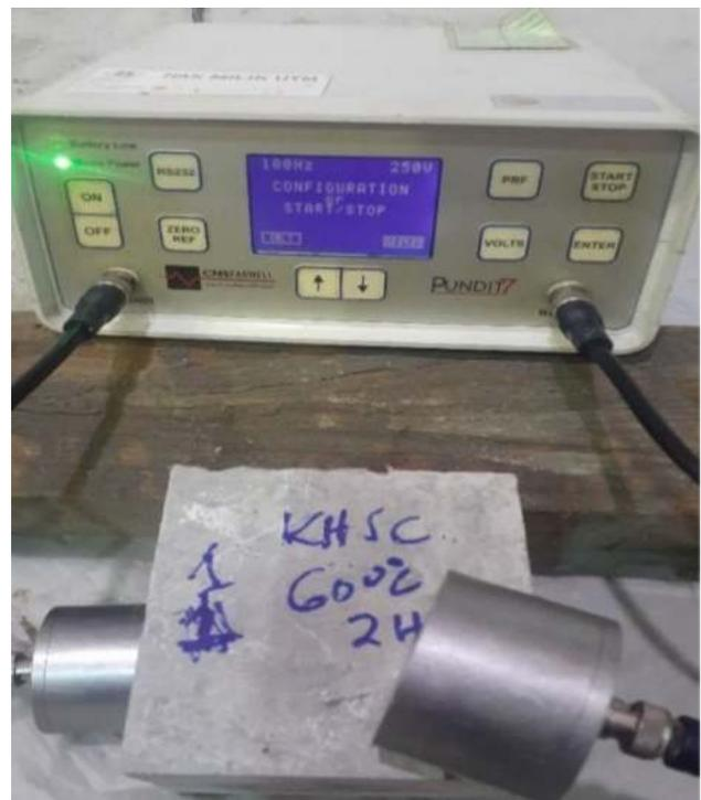
**Fig. 8** The UPV tester for the samples
