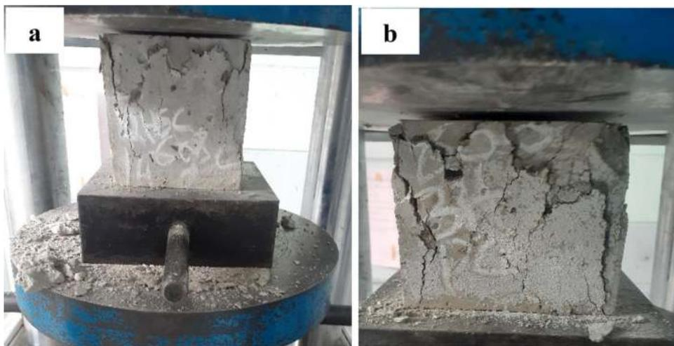
in relative residual strength/strength reduction factor as a function of temperature, which is a much better graph for analysing and comparing changes in strength properties. The strength reduction factor is the residual strength ratio at targeted temperatures to the ambient temperature strength. An example of cubes under crushing load is shown in Fig. 9.
