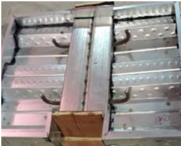
Fig. 18 Embedded toe-to-toe with steel rebar at the sides
