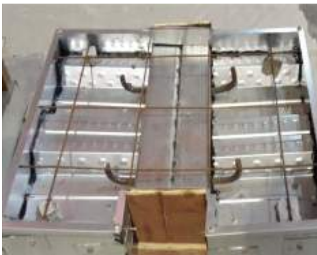
Fig. 9 Specimen No. 6: Steel rebar at the sides
