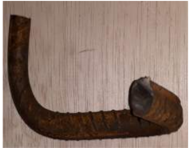
Fig. 19 Steel rebar used as shear connector
