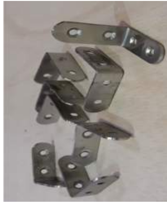
Fig. 23 Brackets used as shear connectors
