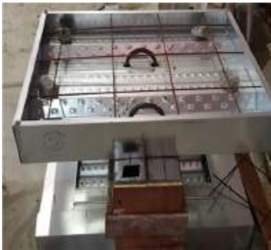
Fig. 8 Specimen No. 5: Steel rebar embedded from the top
