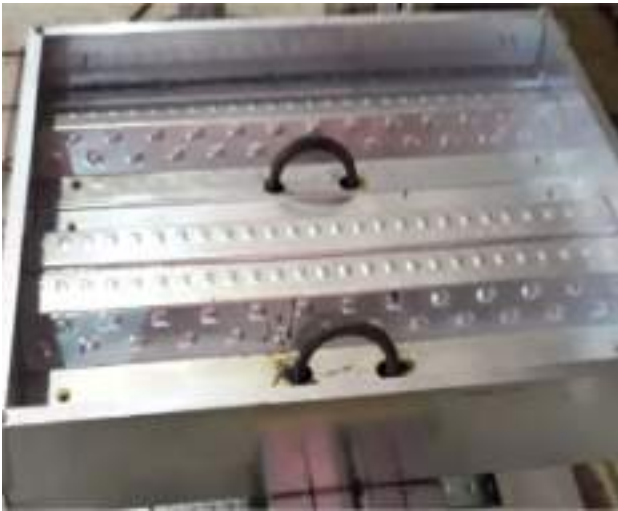
Fig. 21 Steel rebar embedded from the top
