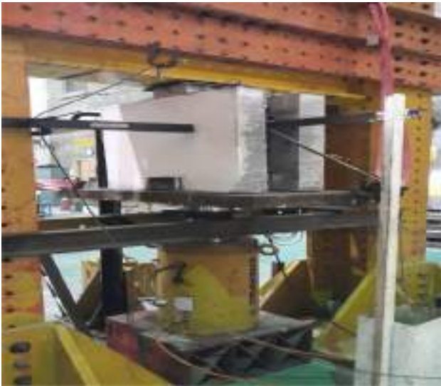
Fig. 25 Set-up of push-out test
