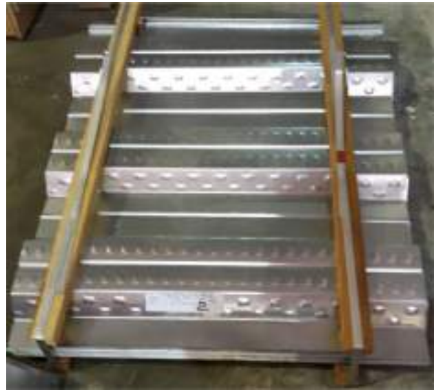
Fig. 27 Metal deck used in the study of 1 mm thick
