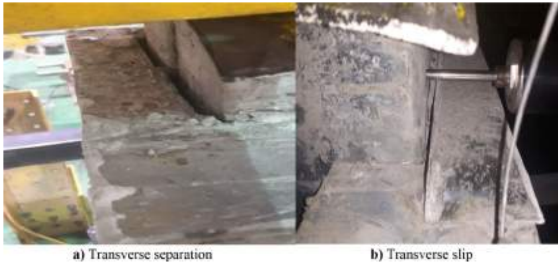
Fig. 45 Transverse separation after test of bent-up tabs specimen. a Transverse separation b Transverse slip
