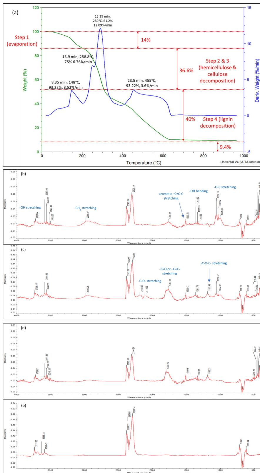
Fig. 5. (a) Thermogravimetric curves of propolis precipitate, (b) FTIR Spectrum at 13.9 min, (c) FTIR spectrum at 16.5 min, (d) FTIR spectrum at 20.9 min and FTIR spectrum at 29.5 min.
