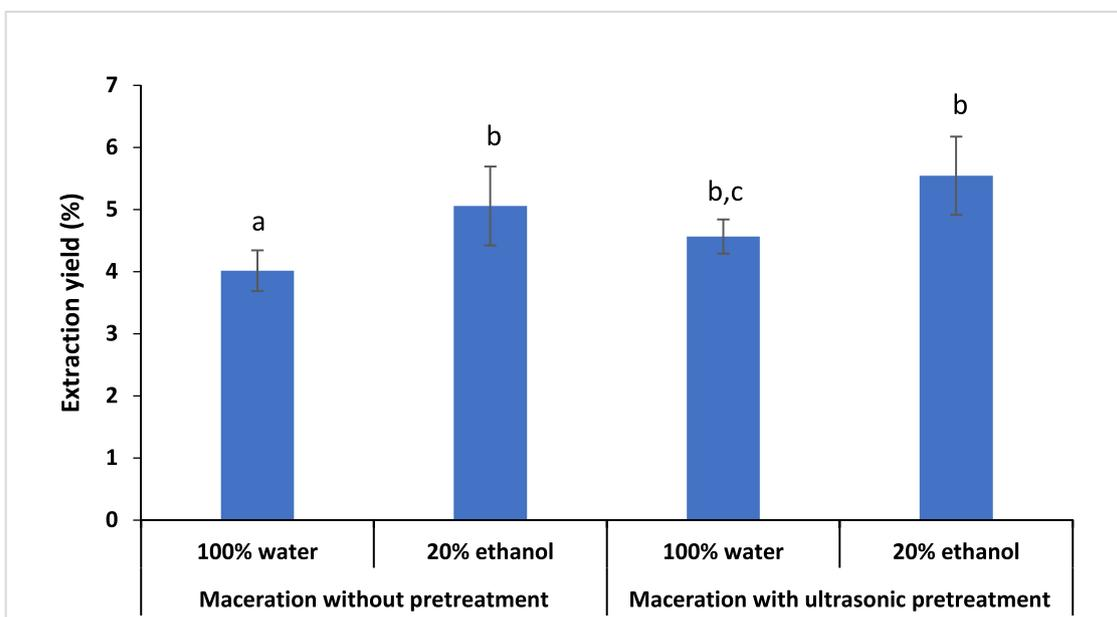
Fig. 2. Yield of propolis extraction using different solvent systems in different extraction technologies such as maceration with and without ultrasonic pretreatment. Different small letters indicate the significant difference of paired two samples for means by T-test
