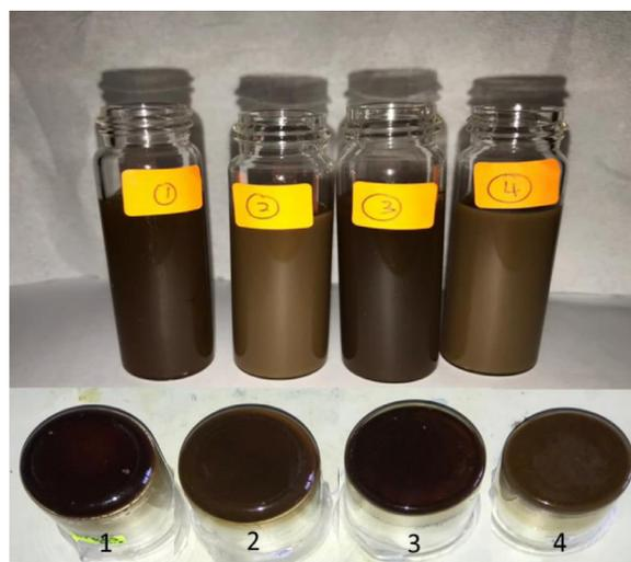
**Fig. 1.** The appearance of concentrated propolis solution and its dried extract, (1) maceration in 100% water, (2) maceration in 20% ethanol, (3) maceration with ultrasonic pretreatment in 100% water and (4) maceration with ultrasonic pretreatment in 20% ethanol.
