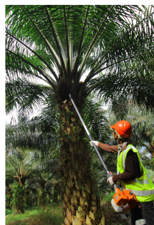
FIGURE 1. CANTAS (engine powered)
