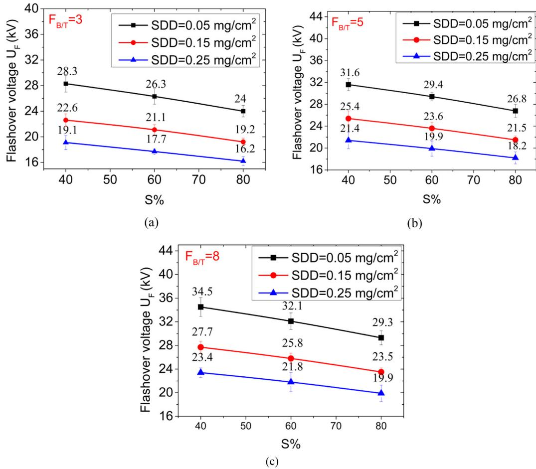
Fig. 7.  $U_F$  of scenario SC-D in term of S%: (a)  $F_{B/T} = 3$ ; (b)  $F_{B/T} = 5$ ; (c)  $F_{B/T} = 8$ .
