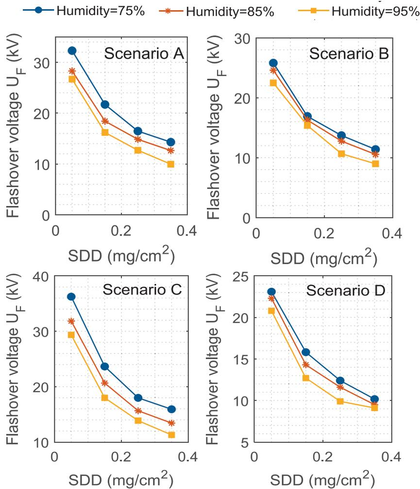
Fig. 4. Flashover voltage versus humidity under studied scenarios.
