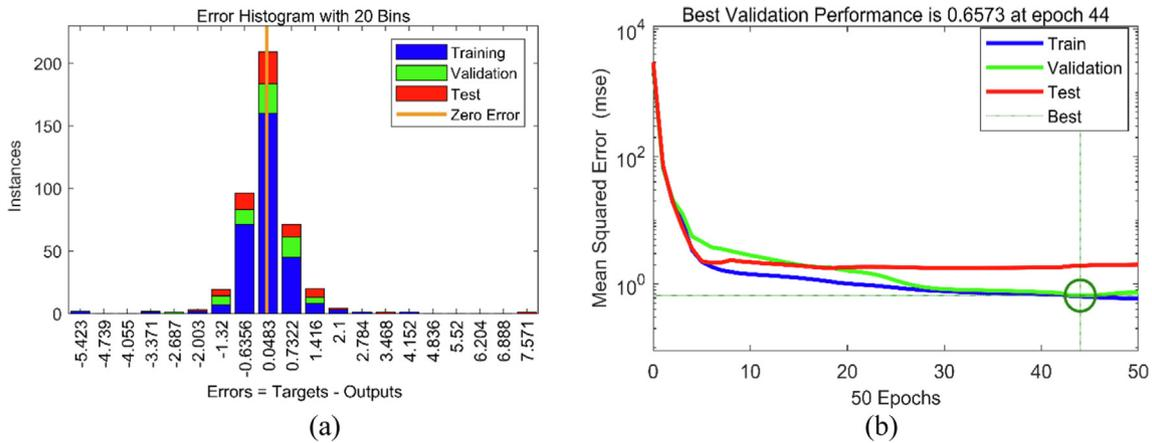
Fig. 9. (a) Artificial neural network error histogram; (b) MSE of trainings, validation and test data.
