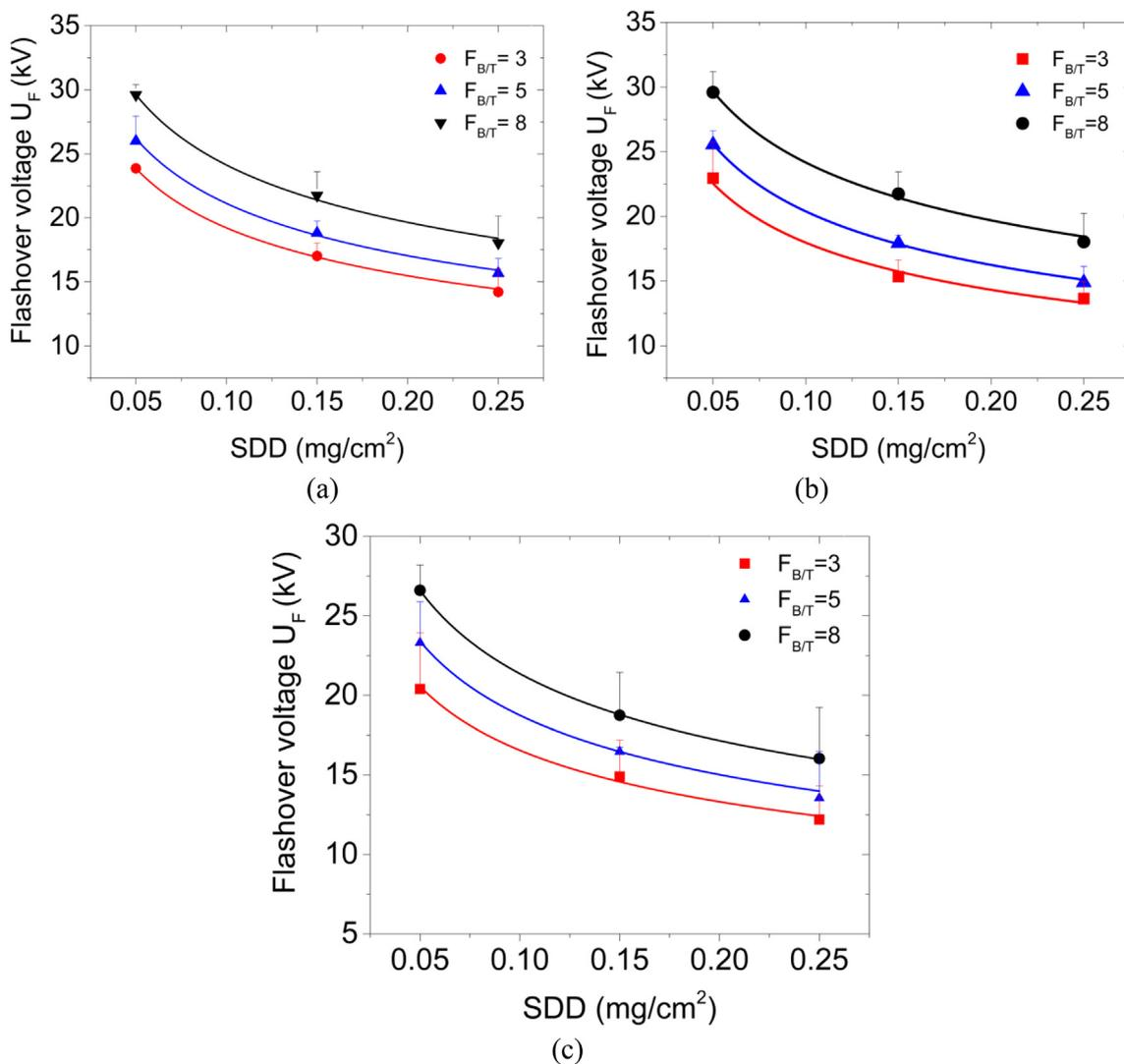
Fig. 5. Non-uniform flashover voltage under S% of 40, 60 and 80%.
