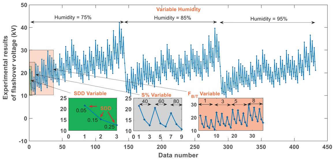
Fig. 8. Experimental results of flashover voltage data under different of SDD, S%,  $F_{B/T}$  and humidity.
