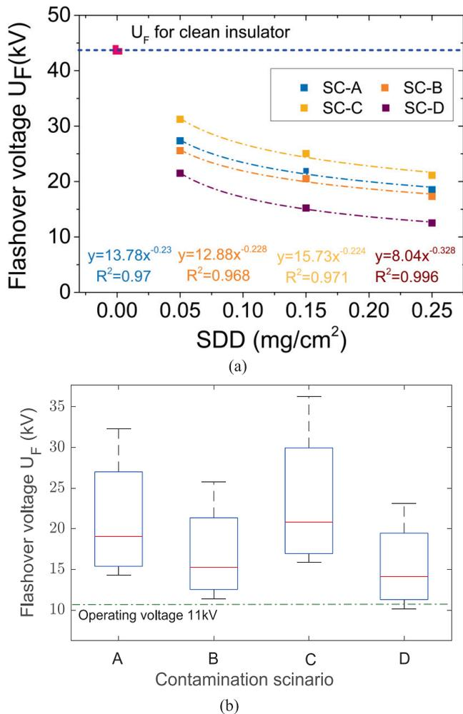
Fig. 3. Studied insulator test results of four scenarios: (a) Relationship between  $U_F$  and  $SDD$ ; (b) Box plot of  $U_F$  for  $SDD$  from 0.05 to 0.25 mg/cm<sup>2</sup>.
