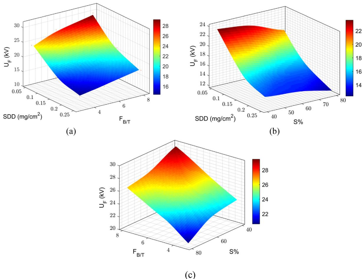
Fig. 6.  $U_f$  of scenario SC-D in term of: (a) SDD and S% at  $F_{B/T} = 3$ ; (b) SDD and  $F_{B/T}$  at  $S\%=40\%$ ; (c) SDD and S% at  $F_{B/T} = 3$ .
