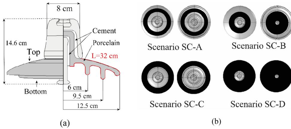
Fig. 1. Test sample: (a) Insulator dimensions; (b) Proposed scenarios of contamination distribution.
