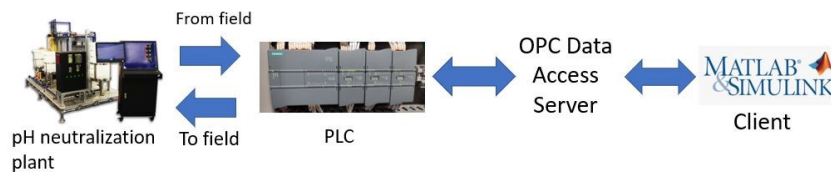
Fig. 4: The network diagram of pH neutralization plant.
