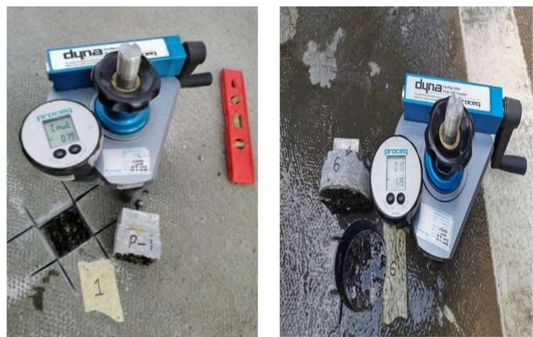
(a) Direct pull-off test
