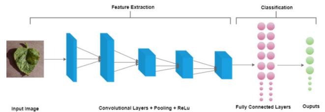
FIGURE 2. Representation of convolutional neural network architecture.
