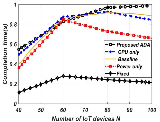
FIGURE 8. Completion time related to number of IoT devices.
