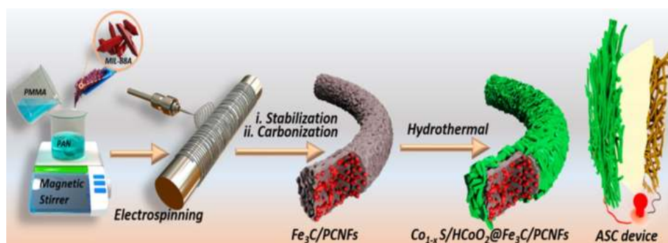
Fig. 1 Schematic diagram of the fabrication process of positive electrode materials for the ASC device
