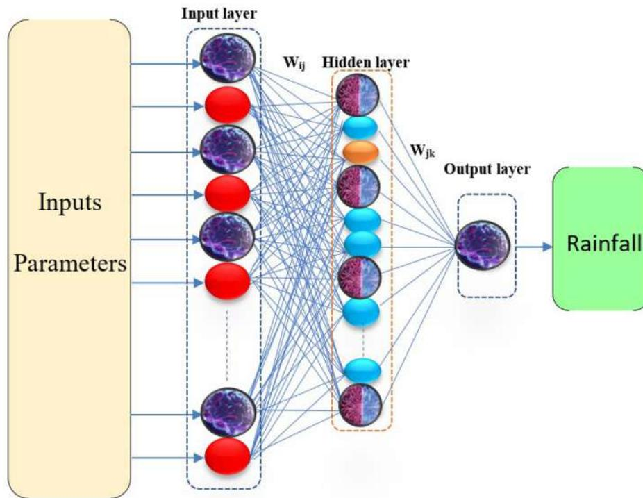
Fig. 4. Structure of FFNN.
