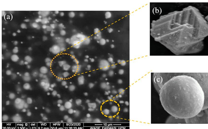
**Fig. 1** – Morphological structure of MRG with  $\text{CoFe}_2\text{O}_4$  under the magnification of  $2500\times$ ; for (a) homogeneous dispersion of both CIPs and  $\text{CoFe}_2\text{O}_4$  particles in the grease medium while, (b) polyhedral shape of  $\text{CoFe}_2\text{O}_4$  and (c) spherical shape of CIP.
