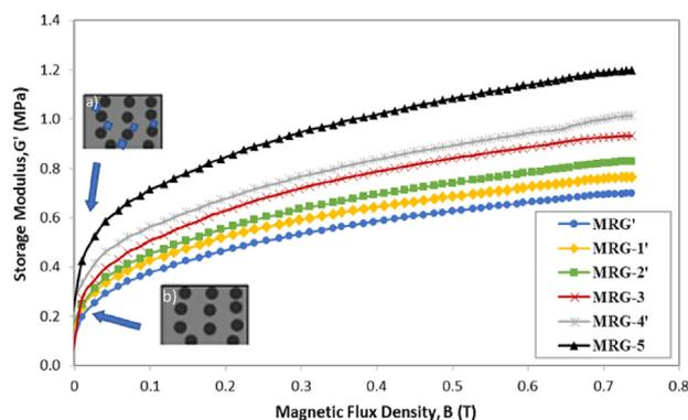
**Fig. 5 – Storage modulus of MRG samples as a function of magnetic flux density from 0 T to 0.75 T. All the MRG samples demonstrated that the storage modulus directly proportional to the magnetic flux density. The schematic illustrations represented the initial structuration of the particles in grease medium which a) with  $\text{CoFe}_2\text{O}_4$  and b) without  $\text{CoFe}_2\text{O}_4$ .**
