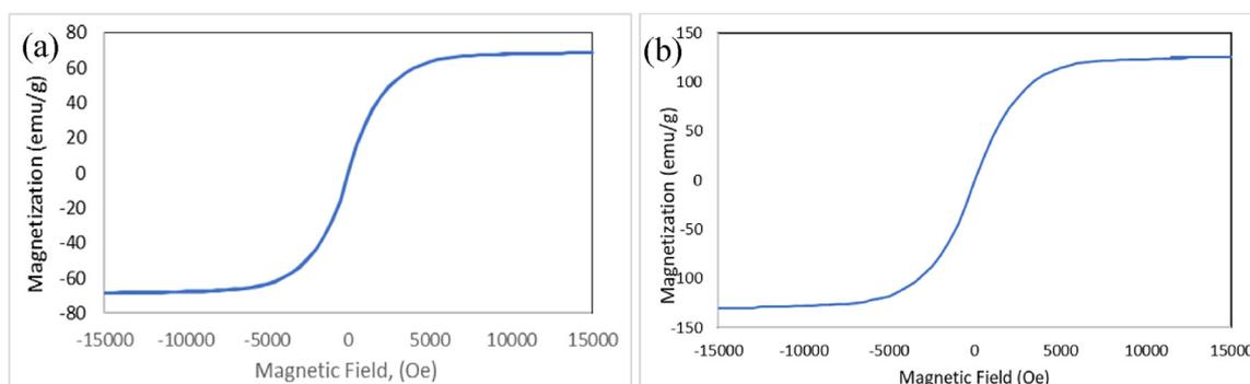
**Fig. 2** – Magnetic hysteresis loop of the particles in this study which (a)  $\text{CoFe}_2\text{O}_4$  recorded the value of magnetization at  $68.8 \text{ emu/g}$  and (b) magnetization of CIP at  $130 \text{ emu/g}$ .
