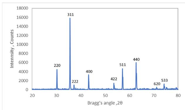
**Fig. 3 – X-ray diffraction of CoFe<sub>2</sub>O<sub>4</sub> from 20° to 80° of Bragg's angle.**
