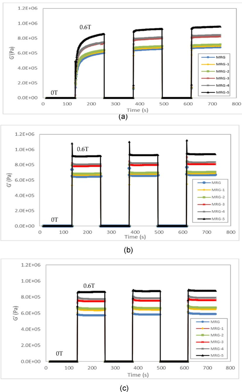
**Fig. 6 – Transient behaviour of MRG samples under different value of applied strains (a) 0.01%, (b) 0.05% and (c) 0.1% when the magnetic field was removed and applied.**
