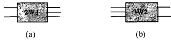
Fig. 6. The symbol for: (a) the 2x3 switch and (b) the 3x2 switch
