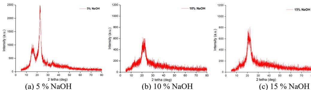
**Figure 2** XRD pattern of treated materials in heating temperature 125 °C with (a) 5 % NaOH, (b) 10 % NaOH, and (c) 15 % NaOH.
