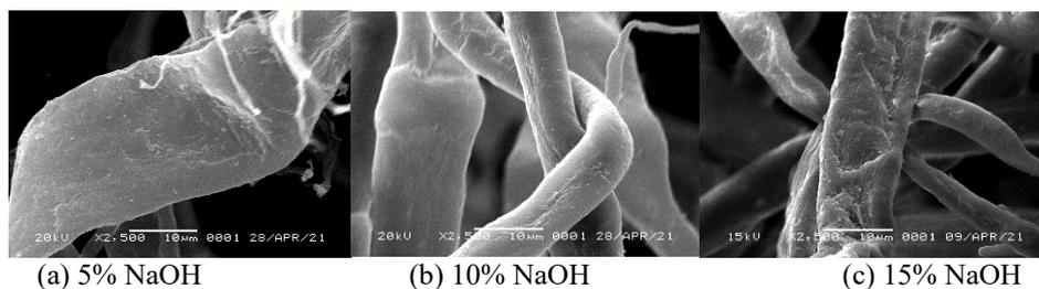
**Figure 7** SEM images of treated waste paper in heating temperature 150 °C with (a) 5 % NaOH, (b) 10 % NaOH, and (c) 15 % NaOH.
