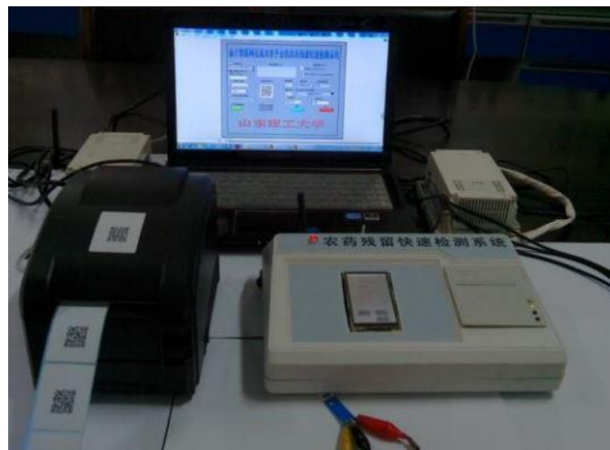
Fig. 11 - The prototype of the detection system [20]
