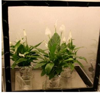
Fig. 9 Small-scale botanical test rig using the peace lily for improving IAQ (Retrieved from Hörmann, Brenske and Ulrichs [22]).
