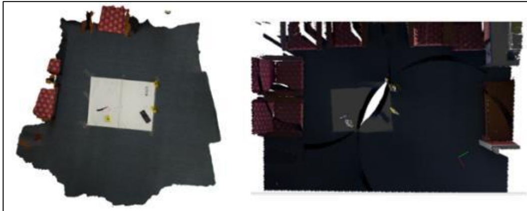
Figure 7. On the left is the output from Micro UAV (Figure 7A) whilst on right is the output from TLS (Figure 7B)
