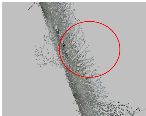
Figure 7. Bullet trajectory at bullet hole 4 and 5. Scanned using BLK2GO Handheld Laser Scanner
