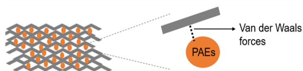
Figure 2. The possible interaction between PAEs and plastic polymers (where the PAEs and plastic polymers were denoted as the orange sphere and grey lines, respectively).
