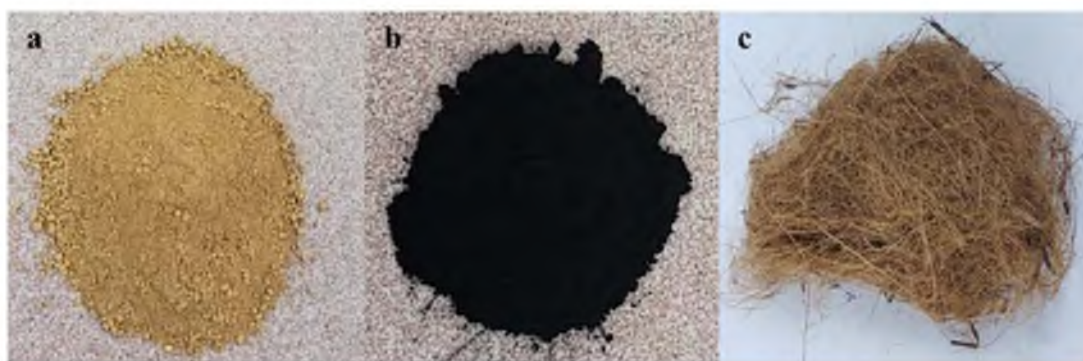
Figure 3. Image of (a) lateritic soil, (b) activated carbon, and (c) coir fibre.
