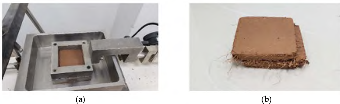
Figure 5. ACF specimen (a) before shearing and (b) after shearing.
