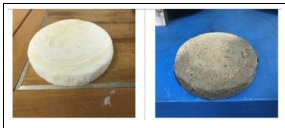
Fig. 7: Conditions of PU foam before and after Rowe Cell consolidation test.
