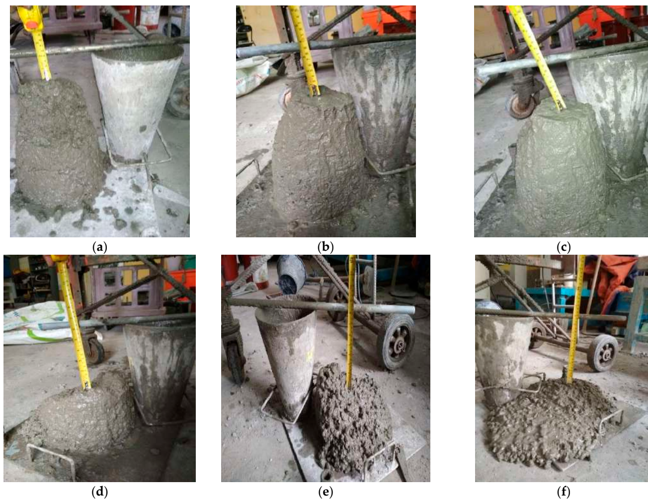
Figure 10. Slump appearance of the concrete mixes with EM of (a) 0%, (b) 5%, (c) 10%, (d) 15%, (e) 20%, and (f) 25%.
