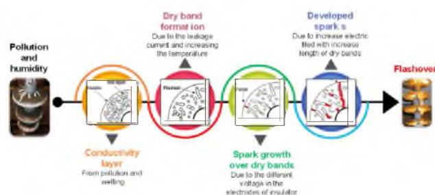
FIGURE 2. Pollution flashover process on an insulator.
