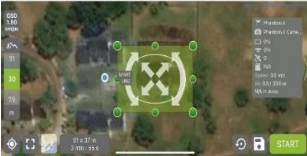
**Figure 7.** Oblique flight planning using Pix4Dcapture software
