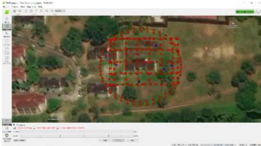
**Figure 13.** Aerial data processing in Pix4Dmapper
