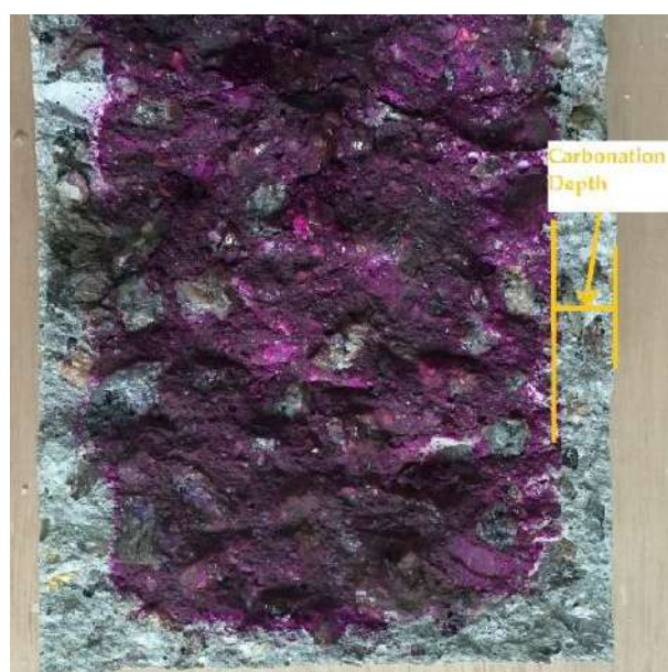
Figure 3. Indication of the depth of carbonation in concrete specimens by using phenolphthalein solution.
