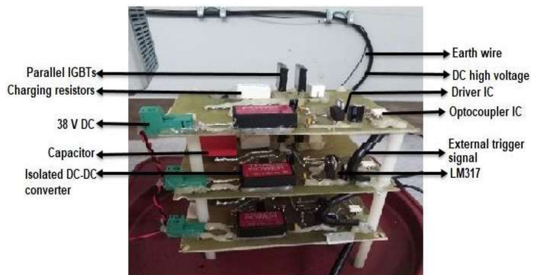
Figure 4. A three-stage Marx generator designed for electroporation.
