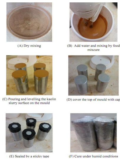
Figure 8. Stage preparation of soil-cement columns.
