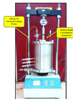
Figure 1. MRCE setup in the TRI-SCAN advance loading frame.
