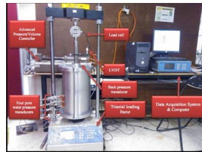
Figure 11. Setup of the MRCE and equipment for the physical testing.
