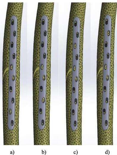
**Fig. 15** Four different types of screw arrangement using 7 screws (a) screw arrangement 1 (b) screw arrangement 2 (c) screw arrangement 3 (d) screw arrangement 4.
