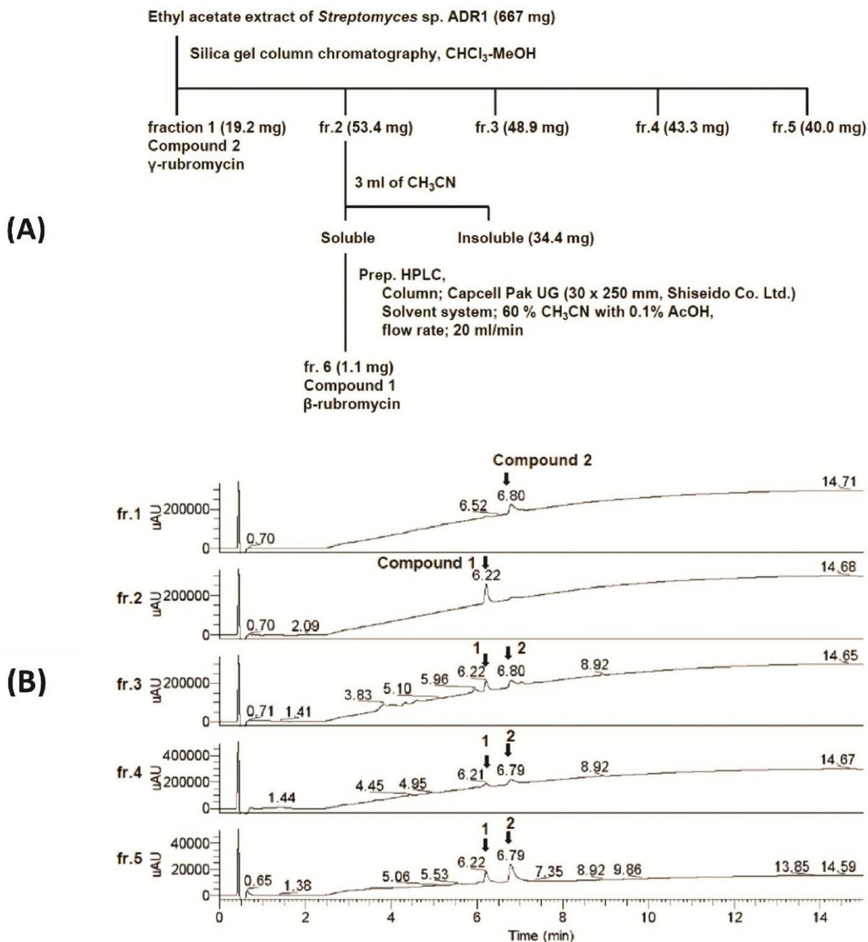
**Figure 4.** (A) Work-up procedure of extraction and purification of β- and γ-rubromycin from *Streptomyces* sp. ADR1; (B) fraction purification by reversed-phase HPLC.
